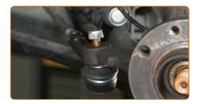
Tighten the lower fasteners connecting the shock strut to the steering knuckle. Use a combination spanner #18. Use a drive socket #18. Use a torque wrench. Tighten it to 105 Nm torque.
