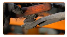
Unscrew the ball joint fastening to the steering knuckle. Use a combination spanner #16. Use a drive socket #16. Use a tap wrench.
