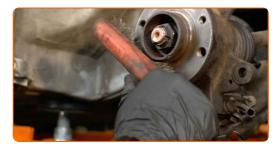
66 Install the brake disc.
