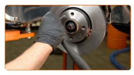
17 Remove the brake disc.
