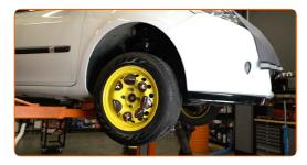
Tighten the drive shaft nut. Use a drive socket #30. Use a torque wrench. Tighten it to 280 Nm torque.
