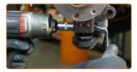
Remove the fastening bolt.
