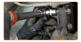
Tighten the fastening nut connecting the tie rod end to the steering knuckle. Use a drive socket #17. Use a torque wrench. Tighten it to 35 nm torque.
