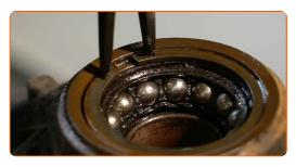
Clean the hub bearing mounting seat. Use a wire brush. Use WD-40 spray.
