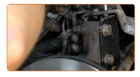
73 Attach the ABS sensor connector.
