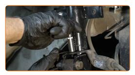
Connect the ABS sensor wiring.
