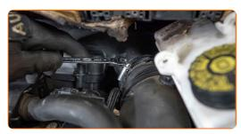
Undo the fastening screws of the air filter cover (3 pieces). Use Torx T25. Use a ratchet wrench.
