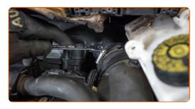
16 Install the brake fluid reservoir.
