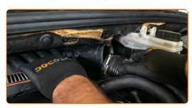
Tighten the clamp and fasteners on the air filter intake pipe. Use a combination spanner #7.
