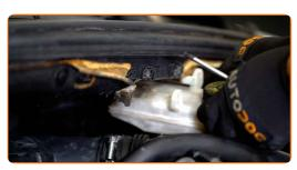
Unscrew the clamp and fasteners on the air filter intake pipe. Use a combination spanner #7.
