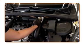
Tighten the brake fluid reservoir fasteners (2 pieces). Use Torx T20.
