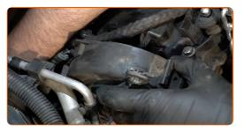
**108** Tighten the fasteners of the upper timing cover. Use a drive socket #10. Use a torque wrench. Tighten it to 12 Nm torque.
