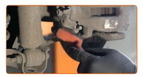
Release the parking brake cable. Use water pump pliers. Use a flat screwdriver.
