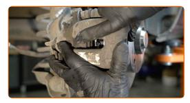
Install the parking brake cable into the brake caliper bracket. Use water pump pliers. Use pliers.
