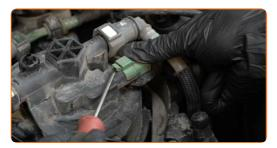
Squeeze the clips and detach the fuel supply lines from the fuel filter housing. Use a flat screwdriver. Use a clip removal tool.
