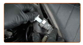
Unscrew the fasteners of the fuel filter housing cover. Use a drive socket #27. Use a ratchet wrench.
