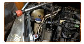
Tighten the engine mount fastening bolts. Use Torx T50. Use a torque wrench. Tighten it to 60 nm torque.
