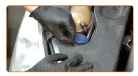
Remove the fender protection cover.
