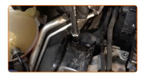
Unscrew the engine mount fasteners. Use Torx T50. Use a ratchet wrench.
