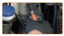
Treat the engine mount fasteners. Use a sealant.
