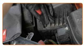
Remove the fender protection cover.
