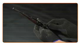
Remove the blade from the wiper arm.
