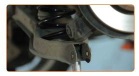
Attach the suspension arm to the rear knuckle. Use a flat screwdriver.
