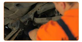
Unscrew the arm fastening to the beam. Use a combination spanner #18. Use a combination spanner #19.
