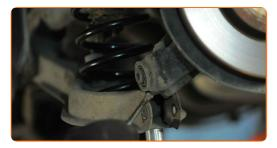
Install the fastening bolt. Use a flat screwdriver. Use a hammer.
