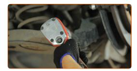
Tighten the arm fastening to the beam. Use a combination spanner #18. Use a combination spanner #19. Use a torque wrench. Tighten it to 103 nm torque.
