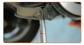
Remove the fastening bolt.
