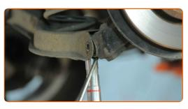
Remove the support from under the stub axle. Use a crowbar.
