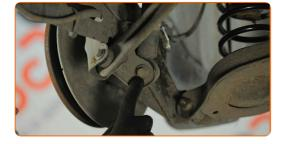
Unscrew the lower fastener of the shock absorber. Use a drive socket #18. Use a ratchet wrench.
