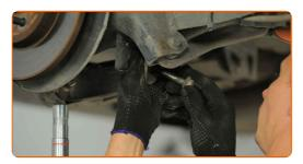
Tighten the lower fastener of the shock absorber. Use a drive socket #18. Use a torque wrench. Tighten it to 120 Nm torque.
