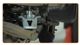
Unscrew the caliper bracket fastening. Use a drive socket #13. Use a ratchet wrench.
