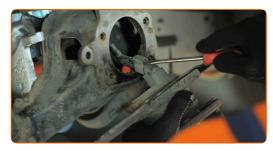
Remove the brake disc cover.
