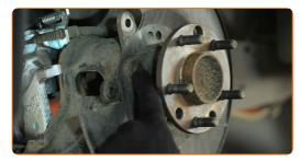
Remove the hub and the bearing together, since they are a sealed unit.
