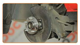
Tighten the hub. Use Torx T50. Use a torque wrench. Tighten it to 70 nm torque.
