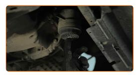
Loosen the drain plug on the oil filter housing. Use HEX No.H5. Use a ratchet wrench.
