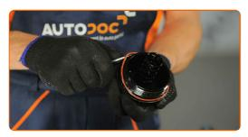
Install a new 0-ring to its mounting seat on the filter cover. Use a flat screwdriver.
