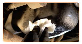
Screw in the new drainage plug and tighten it. Use a drive socket #15. Use a torque wrench. Tighten it to 27 Nm torque.
