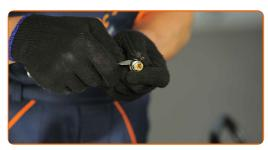
8 Install the new sealing ring. Use a flat screwdriver.
