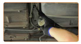
Screw the fixing bolts of the fuel filter bracket. Use a drive socket #8. Use a torque wrench. Tighten it to 9 nm torque.
