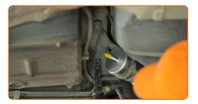
Connect the fuel lines to the fuel filter and lock the fastening clips.
