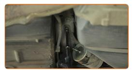
6 Remove the fuel filter together with its bracket.
