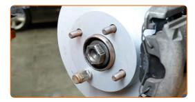
Tighten the drive shaft nut. Use a drive socket #32. Use a torque wrench. Tighten it to 290 Nm torque.
