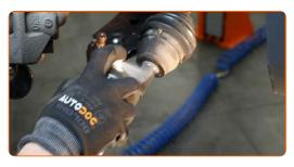
Mount the drive shaft into the wheel hub.
