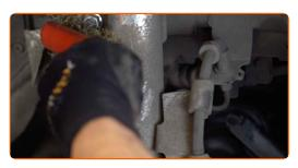
Unscrew the fastener connecting the stabilizer link to the shock strut. Use a combination spanner #17. Use HEX No.H5. Use a ratchet wrench.
