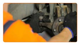
Tighten the fastening nut connecting the tie rod end to the steering knuckle. Use a drive socket #15. Use a torque wrench. Tighten it to 40 nm torque.
