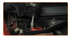
Install the protective shock absorber mounting cap.
