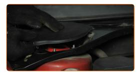
Remove the fender protection cover.
