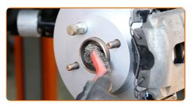
Unscrew the fastener connecting the drive shaft to the wheel hub. Use a drive socket #32. Use a tap wrench.
