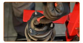
Remove the strut piston rod nut. Use a combination spanner #18. Use HEX No.H6. Use a ratchet wrench.
