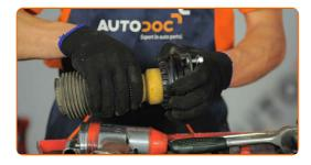
Tighten the shock strut piston rod nut. Use a combination spanner #18. Use HEX No.H6. Use a torque wrench. Tighten it to 58 Nm torque.
