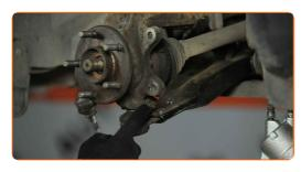
Unscrew the ball joint fastening to the steering knuckle. Use Torx T55. Use a drive socket #18. Use a ratchet wrench.
