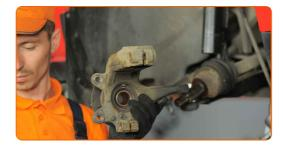
Remove the wheel hub from the steering knuckle. Use a bush and bearing driver set. Use a hammer.
