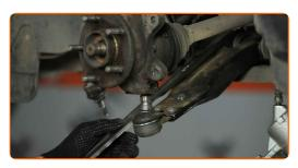
Detach the driveshaft from the steering knuckle.
