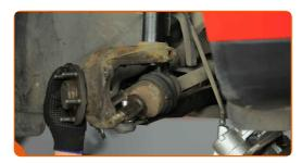
Disconnect the steering knuckle from the shock absorber strut. Use a hammer.
