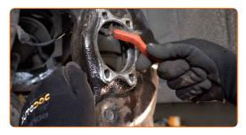
Press the new bearing in the steering knuckle. Use a bush and bearing driver set. Use a hammer.
