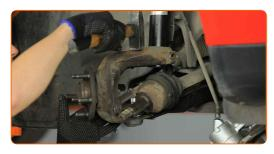
Remove the steering knuckle together with the hub.
