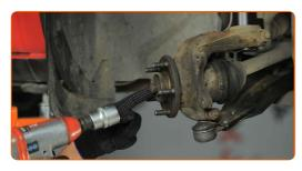
Unscrew the fastener connecting the drive shaft to the wheel hub. Use a drive socket #32. Use a ratchet wrench.
