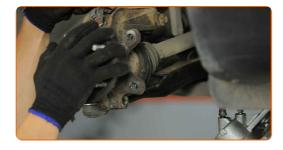
Connect the ball joint to the steering knuckle. Use a crowbar. Use a hammer.
