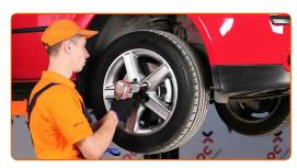
Lower the car and working in a cross order, tighten the wheel bolts. Use wheel impact socket #19. Use a torque wrench. Tighten it to 90 nm torque.
