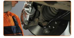
Unscrew the caliper bracket fastening. Use a drive socket #15. Use a ratchet wrench.
