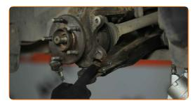
Unscrew the ball joint fastening to the steering knuckle. Use Torx T55. Use a drive socket #18. Use a ratchet wrench.
