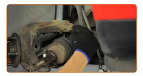
Unscrew the lower fastener connecting the shock strut to the steering knuckle. Use a drive socket #15. Use a ratchet wrench.
