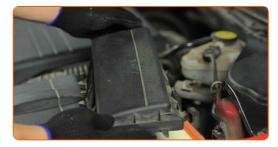
Screw in the fastening screws of the air filter cover. Use a Phillips screwdriver.
