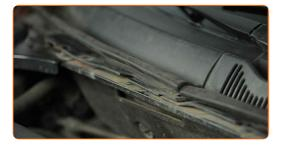
Screw in the fasteners of wiper cowl grille located on the right side. Use Torx T30. Use a ratchet wrench.
