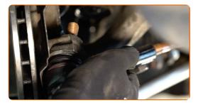
Tighten the fastening nut connecting the tie rod end to the steering knuckle. Use a drive socket #21. Use a torque wrench. Tighten it to 80 nm torque.
