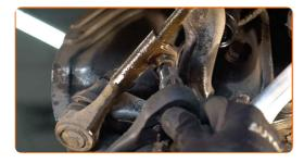
Unscrew the end fastening nut to the steering knuckle. Use a drive socket #21. Use a tap wrench.
