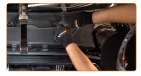
Remove the fender protection cover.
