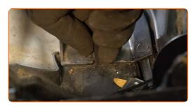
Detach the cable duct from the upper part of the microfilter housing. Use a flat screwdriver.
