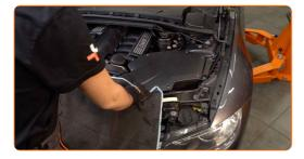
Unscrew the fasteners of the cabin filter housing cover. Use a drive socket #8. Use a ratchet wrench.
