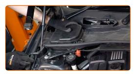
Reinstall the cabin filter housing cover.
