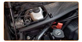
Petach the electrical wiring from the upper part of the microfilter housing.
