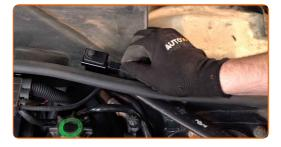
Attach the retainers of the upper part of the microfilter housing.
