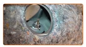
Loosen the upper fastener of the shock absorber. Use a combination spanner #15. Use a drive socket #6. Use a ratchet wrench.
