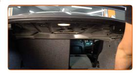
Unscrew the fastener of the central protective plastic panel. Use a clip removal tool. Use a Phillips screwdriver.
