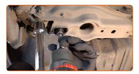
Remove the support from under the arm.
