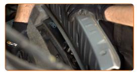
Remove the clips of the boot side lining. Use a clip removal tool.
