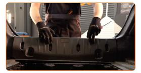
Screw in the fastener of the central protective plastic panel. Use a Phillips screwdriver.
