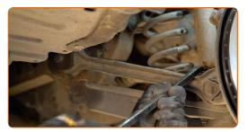
Unscrew the upper fastener of the shock absorber. Use a combination spanner #15. Use a drive socket #6. Use a ratchet wrench.
