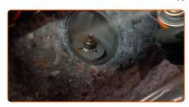
Install the mount cap on the shock absorber upper fastener.
