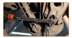
Remove the support from under the arm.
