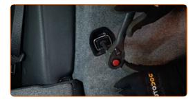
51 Install the clips of the boot side lining.
