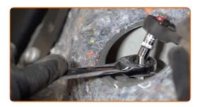
Tighten the lower fastener of the shock absorber. Use a drive socket #17. Use a torque wrench. Tighten it to 60 Nm torque.
