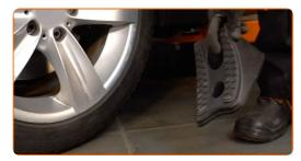
Tighten the top shock absorber fastening. Use a combination spanner #15. Use a drive socket #6. Use a ratchet wrench. Use a torque wrench. Tighten it to 27 Nm torque.
