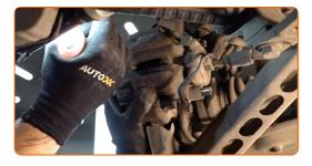
Remove the brake caliper.
