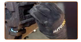
25 Install the brake caliper retaining spring. Use a crowbar.
