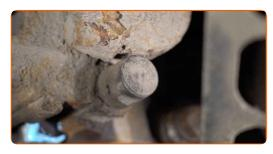
Connect the brake pads wear sensor.
