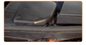
Remove the fender protection cover.
