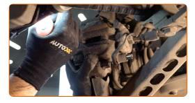
Remove the brake caliper.
