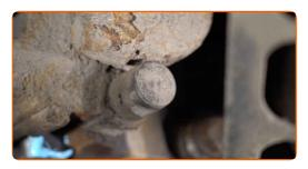
Connect the brake pads wear sensor.
