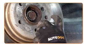
Unscrew the brake disc fastening. Use HEX No.H5. Use an impact screwdriver.
