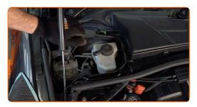
Unscrew the brake fluid reservoir cap.
