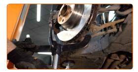
19 Remove the fastening bolt.
