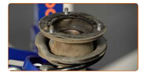
Tighten the shock strut piston rod nut. Use a drive socket #21. Use HEX No.H6. Use a ratchet wrench. Use a torque wrench. Tighten it to 64 Nm torque.
