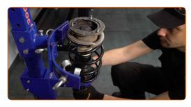
Remove the assembled shock strut.
