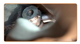
Disconnect the tie rod end from the steering knuckle.
