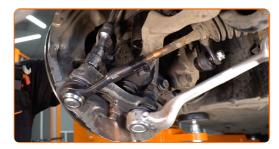
Tighten the lower fasteners connecting the shock strut to the steering knuckle. Use a drive socket #18. Use a torque wrench. Tighten it to 81 Nm torque.
