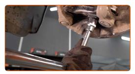
Tighten the fastening nut connecting the tie rod end to the steering knuckle. Use a drive socket #18. Use a torque wrench. Tighten it to 80 Nm torque.
