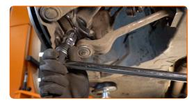
Unscrew the end fastening nut to the steering knuckle. Use a combination spanner #18. Use Torx T30. Use a ratchet wrench.
