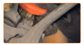
Unscrew the fastener connecting the ball joint of the front control arm to the steering knuckle. Use a drive socket #21. Use a tap wrench.
