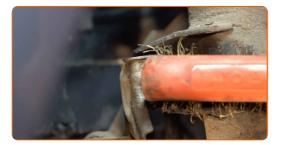
Unscrew the nut and remove the stabilizer rod from the shock strut. Use a drive socket #17.
