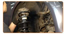
Screw the top fastening of the shock strut mount. Use a drive socket #13. Do not tighten it.
