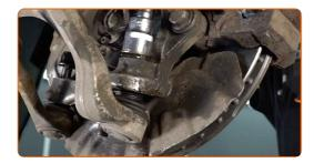
Screw in the fastener connecting the ball joint of the front control arm to the steering knuckle. Use a drive socket #21.
