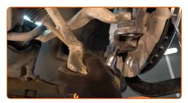
Disconnect the steering knuckle from the shock absorber strut. Use a pin punch. Use a hammer.
