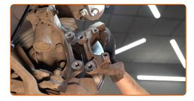
Tighten the brake caliper bracket. Use a drive socket #17. Use a torque wrench. Tighten it to 110 Nm torque.
