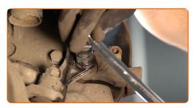
18 Remove the caliper bracket.
