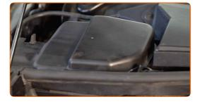
Remove the fender protection cover.
