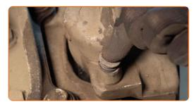
Install the brake caliper retaining spring.
