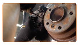
14 Remove the brake caliper.
