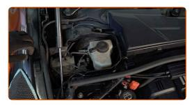
Unscrew the brake fluid reservoir cap.
