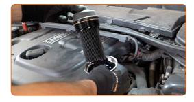
6 Cover the oil filter housing with a microfibre towel to prevent dirt and foreign objects from getting into the system.
