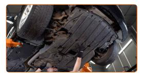
Put a waste oil container with at least 6 l capacity under the drainage hole.
