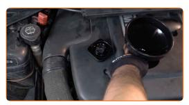
Pour oil into the engine through the filler. Required amount of oil: 5.5 l.
