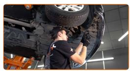
Remove the oil pan cover. Use a drive socket #8. Use a ratchet wrench.
