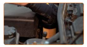
Screw the cap. Use a drive socket #36. Use a torque wrench. Tighten it to 25 Nm torque.
