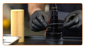
Install the new oil filter to the mounting seat on the filter cover.
