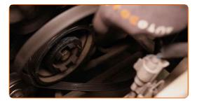
Return the tensioner pulley to its initial position. Use a combination spanner #17. Use a crowbar.
