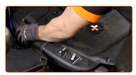
Pull aside the V-ribbed belt tensioner pulley. Use a combination spanner #17. Use a crowbar.
