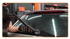
Press the clip. Remove the blade from the wiper arm.
