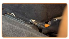
Remove the boot front side lining. Use a crowbar.
