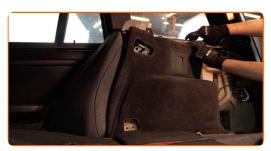
Screw the fasteners of the boot front side lining. Use a Phillips screwdriver.
