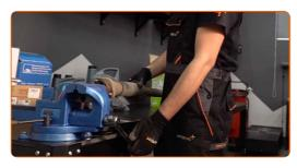
Remove the shock absorber mount, boot and bump stop. 30
