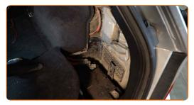
Unscrew the fasteners of the side plastic trim panel. Use Torx T25.
