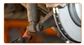
Unscrew the lower fastener of the shock absorber. Use a drive socket #18. Use a tap wrench.
