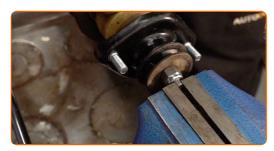
Screw the shock strut piston rod upper fastening. Use a combination spanner #16. Use an adjustable wrench. Use a torque wrench. Tighten it to 20 Nm torque.
