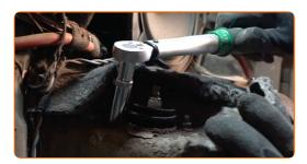
Remove the support from under the arm.
