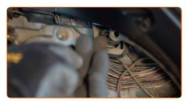
Install the plastic clip of the boot front side lining.
