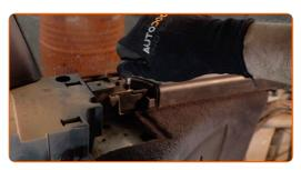
Screw the fasteners of the side plastic trim panel. Use Torx T25.
