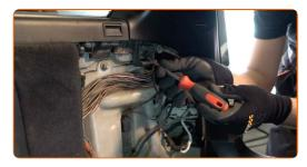
Unscrew the fasteners of the boot front side lining. Use a Phillips screwdriver.
