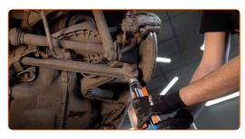
Clean the shock absorber fasteners. Use a wire brush. Use WD-40 spray.
