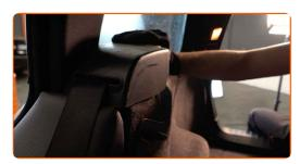
Remove the plastic clip of the boot front side lining. Use a crowbar.
