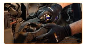
Loosen the upper fastener of the shock absorber. Use a drive socket #13. Use a ratchet wrench.
