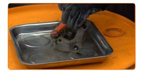
25 Install the brake caliper bracket.
