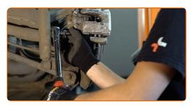
Connect the brake pads wear sensor. Use a crowbar.
