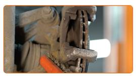
Unscrew the caliper bracket fastening. Use a drive socket #16. Use a ratchet wrench. Use a tap wrench.
