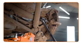
Remove the caliper bracket.
