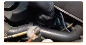
Screw the cap. Use a drive socket #36. Use a torque wrench. Tighten it to 25 Nm torque.
