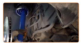
Tighten the fastener connecting the stabilizer link to the shock strut. Use a drive socket #17. Use a combination spanner #17. Use a torque wrench. Tighten it to 55 Nm torque.
