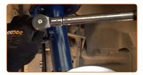
Tighten the fastener connecting the stabilizer link to the stabilizer bar. Use a drive socket #17. Use a combination spanner #17. Use a torque wrench. Tighten it to 55 Nm torque.
