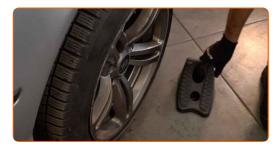
Remove the fender protection cover.
