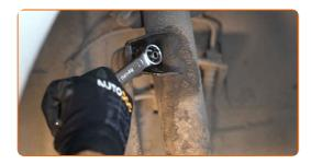
Unscrew the fastener connecting the stabilizer link to the stabilizer bar. Use HEX No.H7. Use a combination spanner #17. Use a ratchet wrench.
