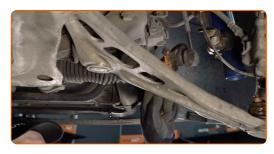
Unscrew the fastener connecting the stabilizer link to the shock strut. Use HEX No.H7. Use a combination spanner #17. Use a ratchet wrench.
