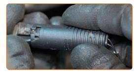
Connect the brake pad wear sensor wire.
