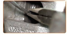
Open the cover of the wiring housing.
