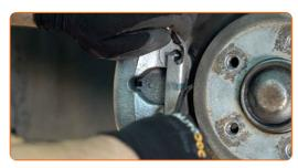
Remove the dust boot caps of the brake caliper guide pins. Use a crowbar.
