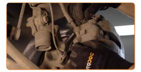
Install the brake caliper retaining spring.
