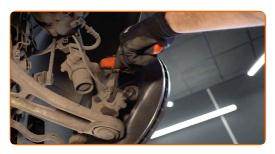
23 Install the brake caliper bracket.
