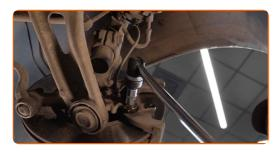
15 Remove the caliper bracket.
