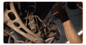
11 Remove the brake caliper.
