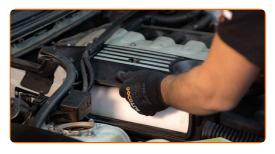
Tighten the oil filler cap.
