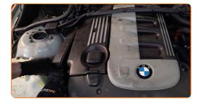
Undo the fastening screws of the air filter cover. Use HEX No.H5. Use a ratchet wrench.
