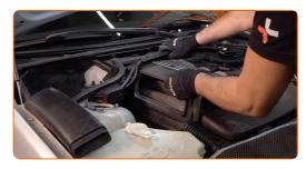
Tighten the oil filler cap.
