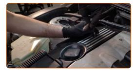
23 Install the air duct housing.
