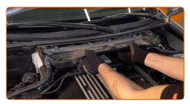
Loosen the air intake fastening. Use HEX No.H5. Use a ratchet wrench.
