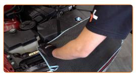
Unscrew the fasteners of the cabin filter housing cover.
