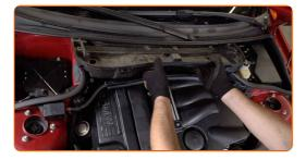
Screw in the cabin filter fasteners. Use Torx T20. Use a ratchet wrench.
