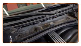
9 Remove the cabin air filter housing.
