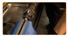
Screw the shock strut piston rod upper fastening. Use a combination spanner #17. Use an adjustable wrench. Use a torque wrench. Tighten it to 20 Nm torque.
