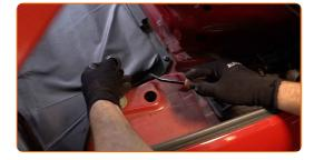
Clean the fasteners of the shock absorber upper mount. Use WD-40 spray.
