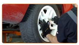
Tighten the top shock absorber fastening. Use a drive socket #13. Use a torque wrench. Tighten it to 28 Nm 33 torque.
