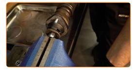
Screw the shock strut piston rod upper fastening. Use a combination spanner #17. Use an adjustable wrench. Use a torque wrench. Tighten it to 20 Nm torque.
