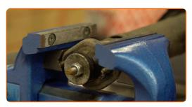
Clean the shock absorber rod fastener. Use a wire brush.
