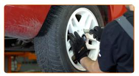
Tighten the top shock absorber fastening. Use a drive socket #13. Use a torque wrench. Tighten it to 28 Nm torque.
