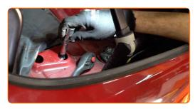
Tighten the lower fastener of the shock absorber. Use a drive socket #18. Use a torque wrench. Tighten it to 100 Nm torque.
