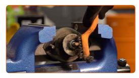
Remove the shock absorber piston rod fastening. Use a combination spanner #17.
