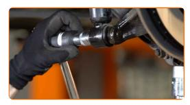
Remove the fastening bolt.
