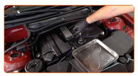
Screw the cap. Use the 86/16 F socket. Use a torque wrench. Tighten it to 25 Nm torque.
