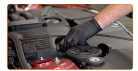
Pour oil into the engine through the filler. Required amount of oil: 5.5 L.
