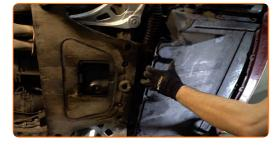
Screw in the fasteners of the lower sound insulation. Use a Phillips screwdriver.
