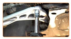
Tighten the arm fastening to the subframe. Use a combination spanner #21. Use a torque wrench. Tighten it to 90 nm torque.
