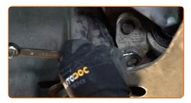
Insert the ball joint into the steering knuckle and fix it with a new nut.
