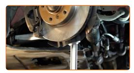
Tighten the ball joint fastening nut. Use a combination spanner #19. Use a torque wrench. Tighten it to 65 nm torque.
