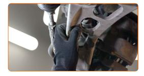
Unscrew the arm fastening from the subframe. Use a combination spanner #21.
