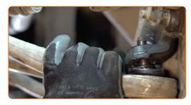
Disconnect the lower arm from the steering knuckle.
