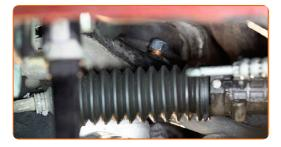
Screw the fastener connecting the control arm to the subframe. Use a combination spanner #21.
