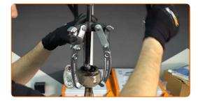
Loosen the vice and remove the control arm.
