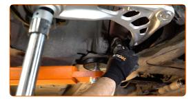
Remove the support from under the arm.
