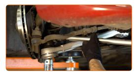
Tighten the rear fastener of the control arm. Use a drive socket #18. Use a combination spanner #18. Use a torque wrench. Tighten it to 59 nm torque.
