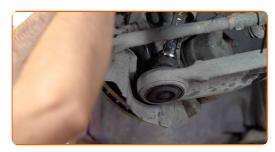
Detach the fastener connecting the suspension level sensor to the suspension control arm. Use a drive socket #13. Use a ratchet wrench.
