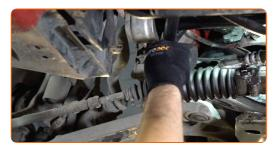
Unscrew the rear arm fastening. Use a drive socket #18. Use a combination spanner #18. Use a ratchet wrench.
