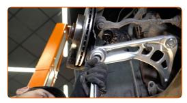
Screw the fastener connecting the ball joint to the steering knuckle. Use a combination spanner #19.
