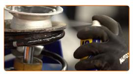
Tighten the shock strut piston rod nut. Use a drive socket #22. Use HEX No.H7. Use a torque wrench. Tighten it to 64 Nm torque.
