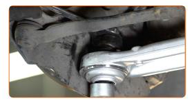
Tighten the lower fasteners connecting the shock strut to the steering knuckle. Use a drive socket #21. Use a torque wrench. Tighten it to 80 Nm torque.
