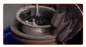
Remove the strut piston rod nut. Use a drive socket #22. Use HEX No.H7.
