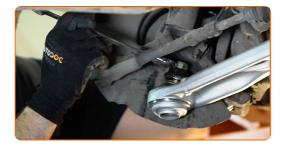
Unscrew the lower fastener connecting the shock strut to the steering knuckle. Use a drive socket #21. Use a tap wrench.
