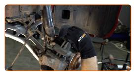
Unscrew the shock absorber mount fastening. Use a drive socket #13. Use a ratchet wrench.
