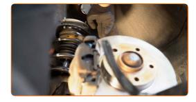
Secure the upper fasteners of the shock strut. Use a drive socket #13. Do not tighten it.
