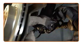
Install and tighten a new bolt of the steering knuckle.
