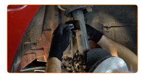
Unscrew the ball joint fastening to the steering knuckle. Use a combination spanner #19.
