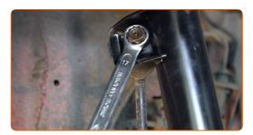
Tighten the ball joint fastener. Use a combination spanner #19. Use a torque wrench. Tighten it to 65 Nm torque.
