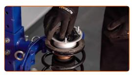
Remove the assembled shock strut.
