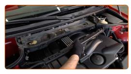
Unscrew the filter housing fastening bolts. Use Torx T20. Use a ratchet wrench.
