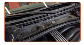
9 Remove the cabin air filter housing.
