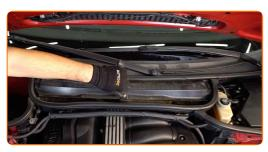
18 Remove the fender protection cover.
