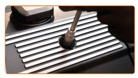
Install the engine cover and secure it.
