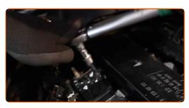
Treat the ignition coil connector with electronic spray.
