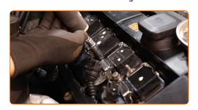
Take out the ignition coils from the spark plug wells. 13
