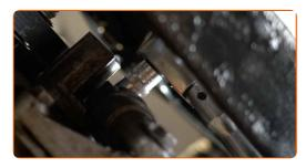
Screw in the fastener of the AC compressor belt tensioner pulley. Use a drive socket #13. Use a torque wrench. Tighten it to 7 Nm torque.
