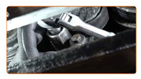
Remove the AC compressor belt.
