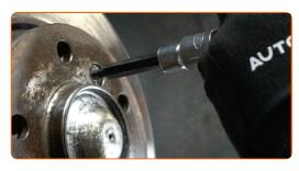
Remove the brake disc.
