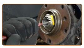
Unscrew the hub nut. Use a drive socket #46. Use a tap wrench.
