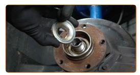
Remove the wheel hub together with the bearing. Use 3-Arm Gear Puller.
