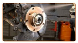
Install the cap of the hub nut. Use a drive socket #46. Use a hammer.
