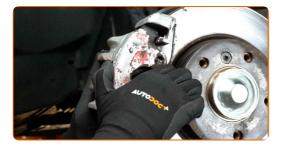
Tighten the brake caliper bracket. Use a drive socket #16. Use a torque wrench. Tighten it to 110 Nm torque.
