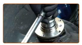
Restake the wheel hub retaining nut. Use a flat metal-working chisel. Use a hammer.
