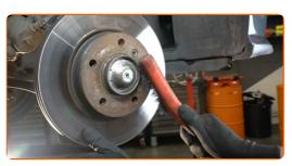
Unscrew the brake disc fastening. Use HEX No.H6. Use an impact screwdriver.
