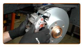
19 Install the brake caliper retaining spring.
