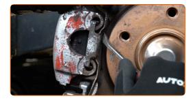
11 Remove the brake caliper.
