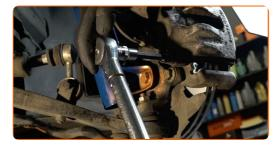
21 Install the dust boot caps of the brake caliper guide pins.
