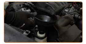
Pour coolant in the coolant reservoir.
