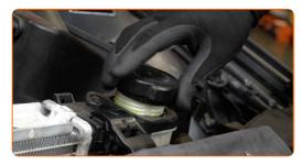
Screw on the coolant reservoir cap.
