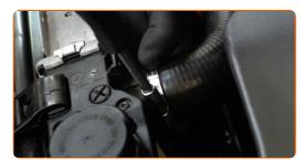
Remove the coolant reservoir cap.
