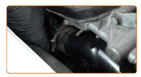
Fasten the clamps of the coolant hoses. Use a drive socket #7. Use a ratchet wrench.
