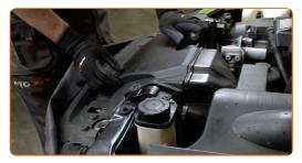
Install the air duct housing fasteners.
