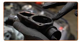
Install the new thermostat housing.
