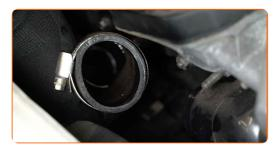
Detach the coolant pipe bracket. Use a drive socket #13. Use a ratchet wrench.
