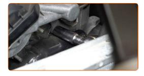
Unscrew the thermostat housing fasteners. Use a drive socket #10. Use a ratchet wrench.
