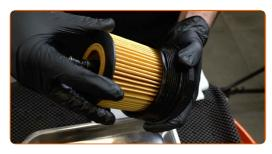
Install a new O-ring to its mounting seat on the filter cover.
