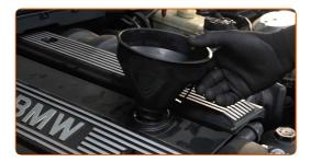
Pour oil into the engine through the filler. Required amount of oil: 6,5 l.
