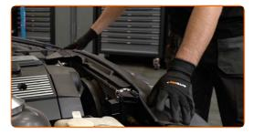
Release the air filter cover clips.
