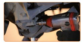
Remove the support from under the arm.
