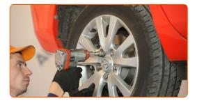
Lower the car and working in a cross order, tighten the wheel bolts. Use wheel impact socket #19. Use a torque wrench. Tighten it to 118 nm torque.
