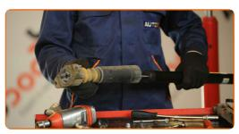
Tighten the shock absorber mount fasteners. Use a combination spanner #13. Use an adjustable wrench. Use a torque wrench. Tighten it to 25 nm torque.
