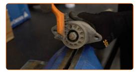
Unscrew the shock absorber mount fasteners. Use a combination spanner #13. Use an adjustable wrench.
