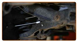
Treat the shock absorber fasteners. Treat all joints of the arm. Treat all joints of the stabiliser link. Use copper grease.
